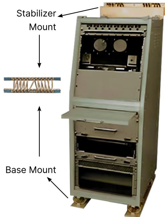
Shown above is an application for ground transport, airframe, or shipboard installation. Not only does this arrangement dampen shock and vibration in three axes, but it also allows designers/engineers to use COTS equipment rather than the more expensive ruggedized electronic equipment.
