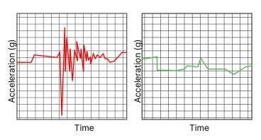
Input Shock versus Damping
